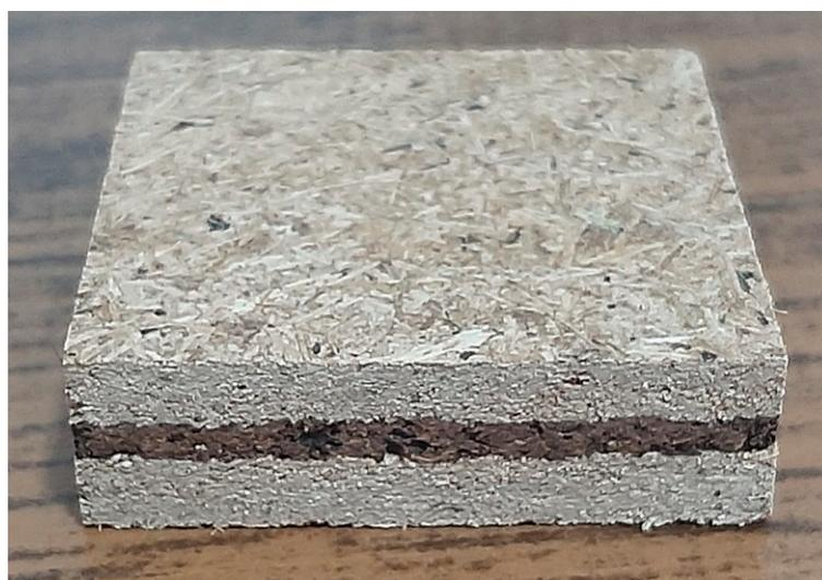
**Figure 1.** Sugarcane bagasse and sargassum particleboard sample (50 × 50 mm).
