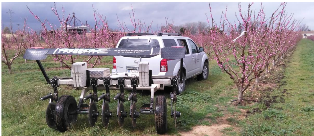
Figure 1 Study plot and Veris 3100 soil sensor for ECa surveying.
