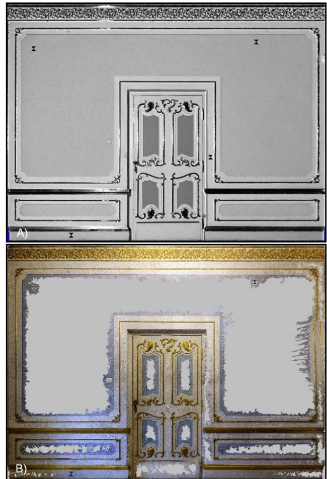
Figure 4. A) Orthoimage from reflectance intensity. B) Orthoimage generated based on the point cloud from image matching.
