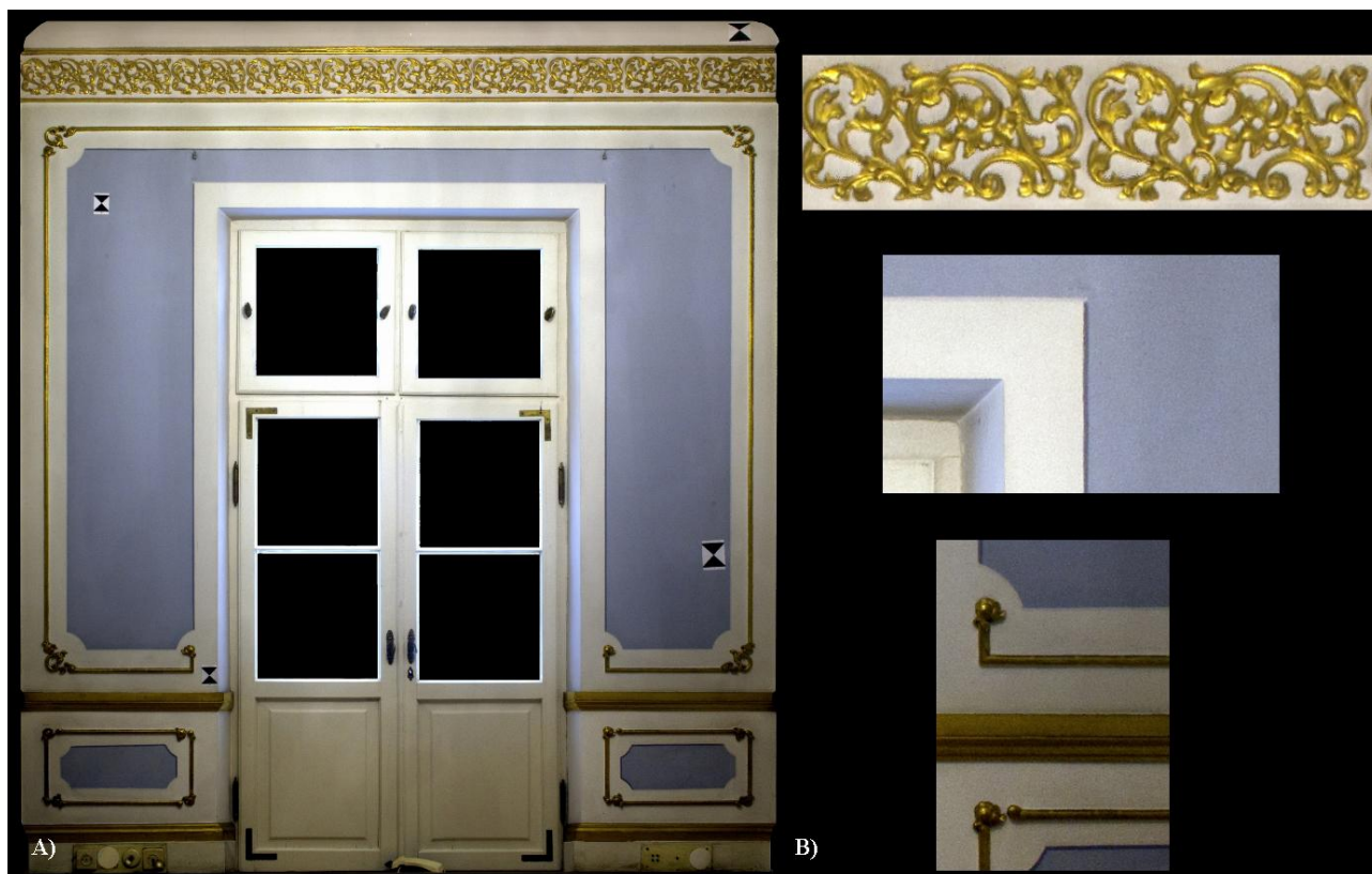
Figure 9. A) An orthoimage generated from integration of point clouds from TLS and image matching. B) Zooms show selected elements of the processed wall.
