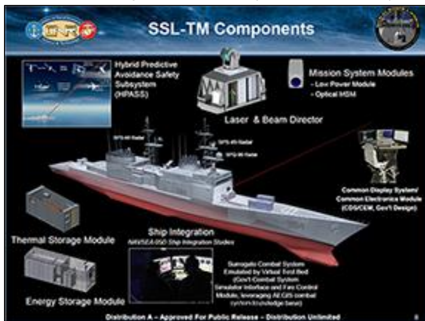
Figure 5. ONR Graphic of SSL-TM Laser System Artist's rendering of installation on Navy's Self Defense Test Ship
