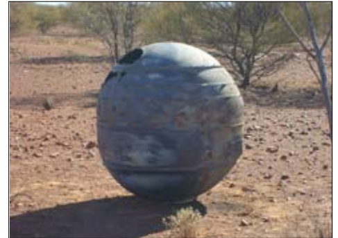
Figure 1. A solid rocket motor casing from a commercial U.S. Delta 2 launch vehicle was found in Australia, nearly 18 years after it reentered.
