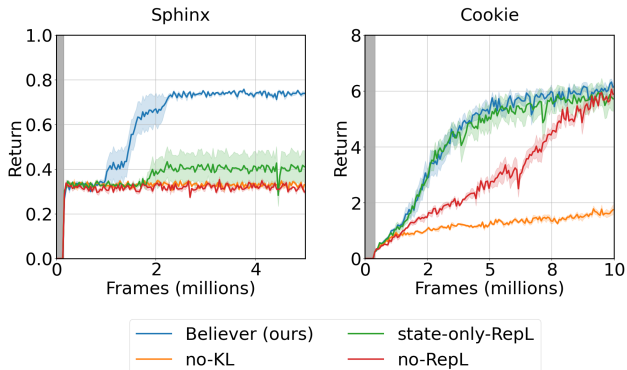
Figure 8. We conduct ablations to verify the design choices in Believer. The figure shows return per episode plotted over the course of training (measured in total training frames), averaged over five seeds, with shaded bars showing standard error and the shaded grey area representing the pretraining dataset size. Representation learning and applying an information bottleneck are critical for performance and/or sample efficiency. Discarding observable features from the state encoding is critical in Sphinx.
