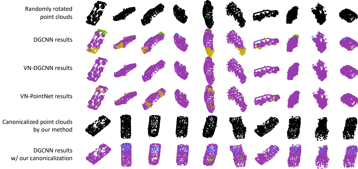
Figure 9. Qualitative visualization of part segmentations of our method (car, I/SO(3) ) on the ShapeNet dataset.
