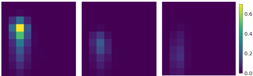
Figure 5: The average 10 \times 10 persistence image constructed from the persistence diagram of the 1-dimensional homology for each temper condition: (left) “as extruded”; (middle) T5; (right) T6.
