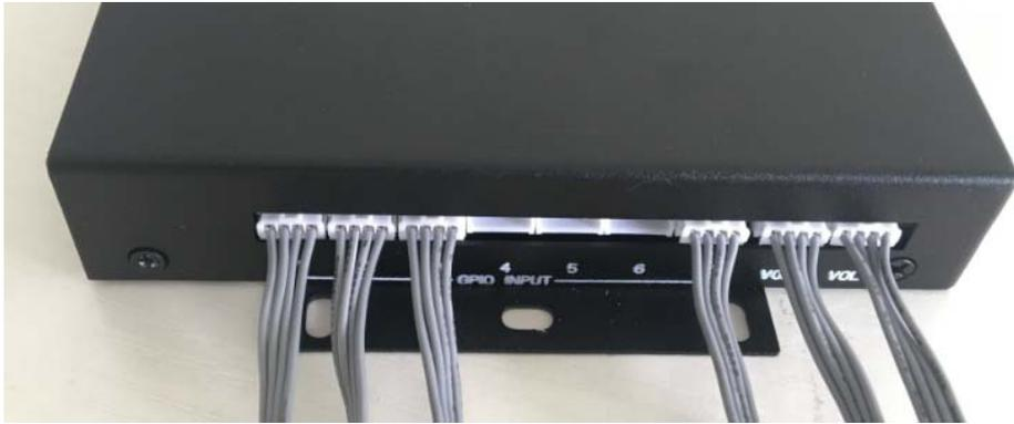
Connect Push buttons in GPIO 1#,2#,3#,7#, and V+, V-
