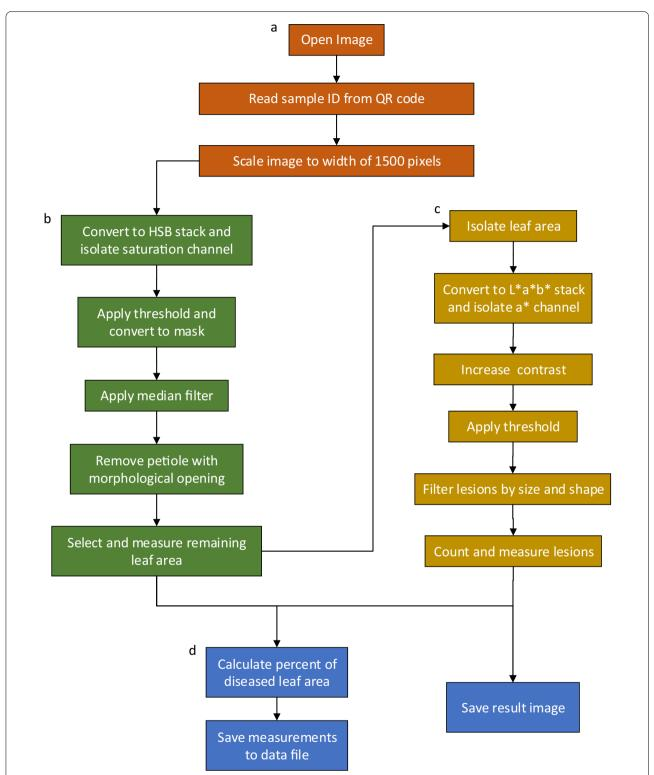
**Fig. 1** A method for measuring and counting frogeye leaf spot lesions on soybean leaves. The four main steps are **a** image preprocessing, **b** leaf segmentation, **c** lesion segmentation, and **d** calculation and data reporting
