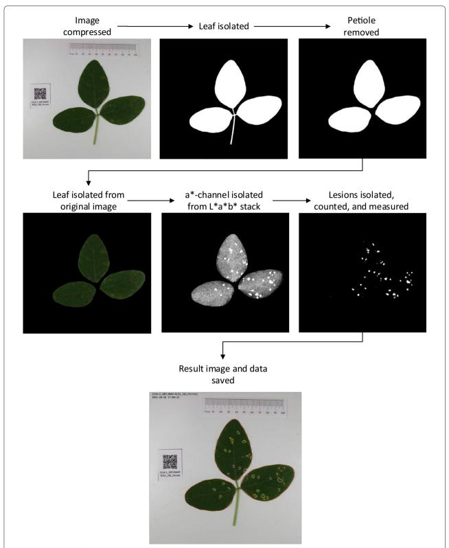
Fig. 4 Image processing first isolates the leaf, removes the petiole, and measures the leaf. From the leaf, it then isolates, measures, and counts the lesions
