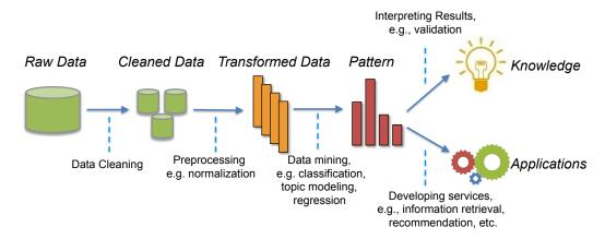
Figure 1.2: A Process of Data Mining
