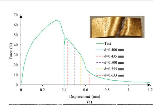
(a) Force–displacement and (b) damage evolution of the paper–Al laminate subjected to uniaxial tensile loading. Credit: *ACS Omega* (2024). DOI: 10.1021/acsomega.4c05798
