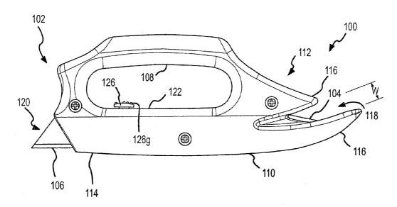
(57) Abstract: The present invention provides a dual blade utility knife useful in various fields. In particular, the dual blade utility knife contains a fixed cutting element contained in a gap that inhibits injury or accidents, a.k.a. a safety knife. The second cutting element is designed to be retractable. The retractable blade can be retracted during use of the safety blade, inhibiting injury or accidents, but extended to make cuts, such as an initial cut in a material.
