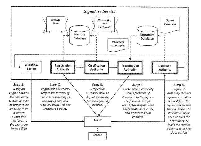
FIG. 1 System for Signing and Authenticating Electronic Documents
