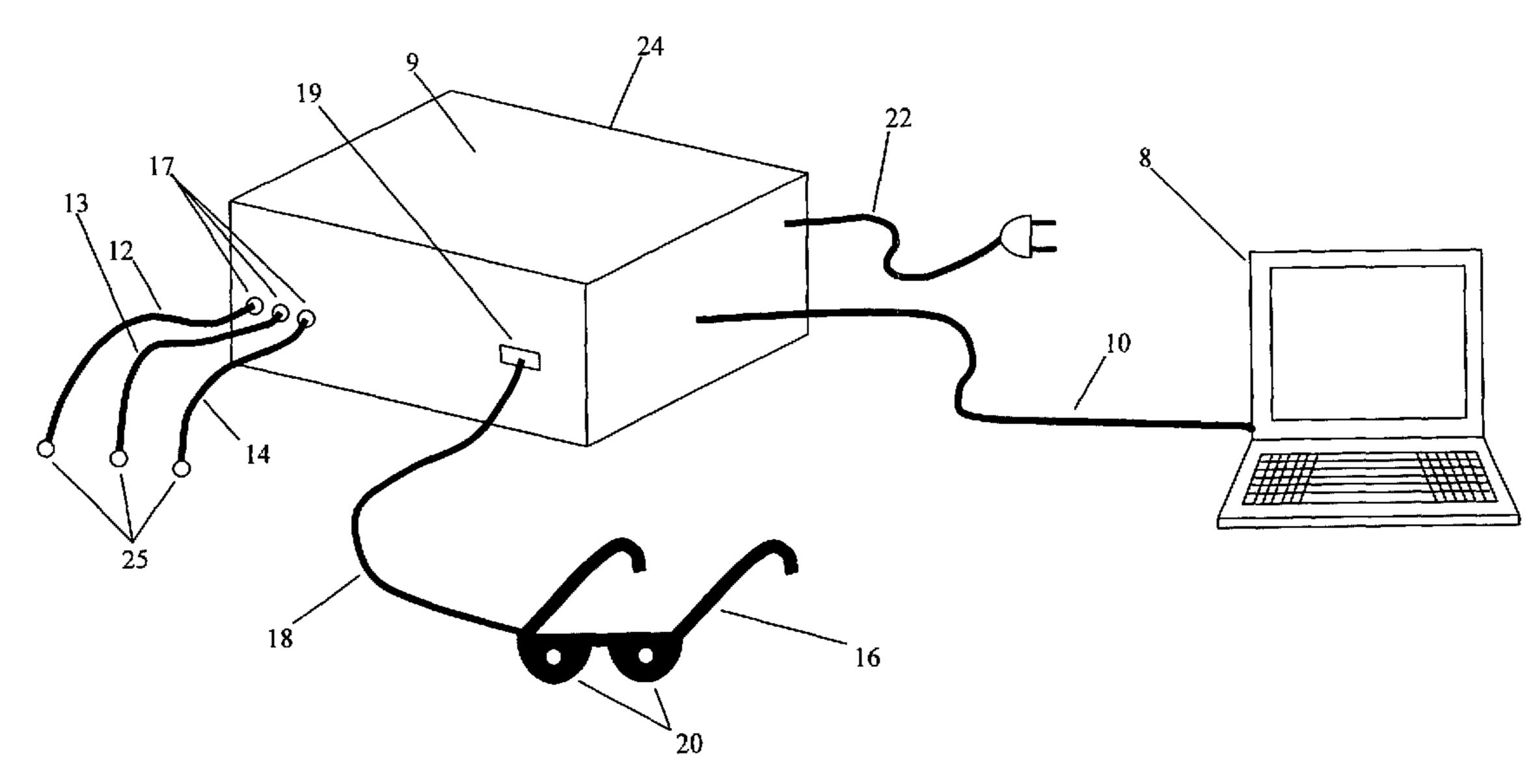
(57) Abstract: A computing device-controlled system (8) is described for the generation of amplitude-modulated pulse-width modulation signals for use in treating neurological dysfunction via cranial neurostimulation.
