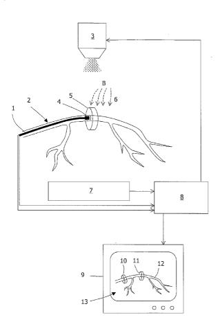
(57) Abstract: The invention relates to an apparatus and a method for the joint three-dimensional display of an angiogram (12) and local intravascular images (10, 11). The angiogram (12) is preferably recorded by means of an X-ray apparatus (3, 7), while the local intravascular images are generated by an ultrasound probe (4) on a catheter (1). The position of the probe (4) is determined by a position determination unit and is used to assign the recorded volume (5) to the angiogram (12).
