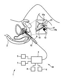
imaging unit (4) generates an indicator image showing the inner part (19) and an indicator of the introduction element (17) based on the tracked location. A display (5) displays the indicator image providing feedback about the location of the introduction element (17).
