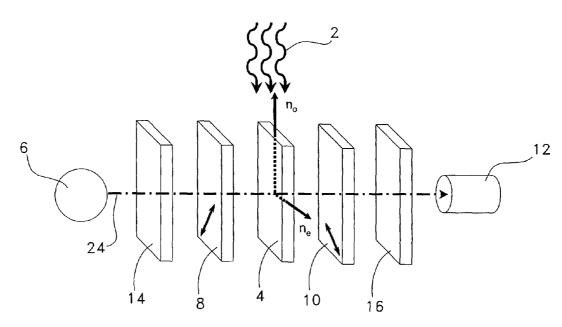
(57) Abstract: A method and a sensor for detecting a chemical substance in an analyte. An anisotropic material is subjected to the analyte. Light is passed through the anisotropic material and collected. A change of an optical anisotropy of the collected light is detected, the change being indicative of the chemical substance in the analyte.
