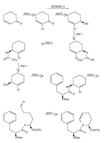
In Scheme A step a, cyclohexenone is sequentially con- $_{50}$  tacted with an appropriate chlorinating agent and an appropriate base to give 2-chlorocyclohex-2-en-1-one.
