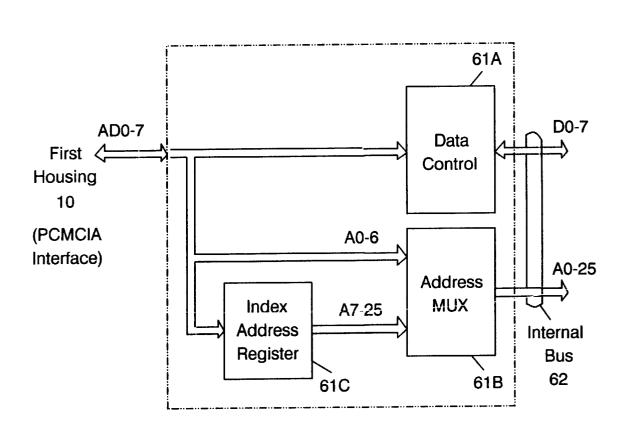
FIG. 5 A7-14 Offset 0 Offset 1 A15-22 A23-25 Offset 3 **Index Address Register** 61C
