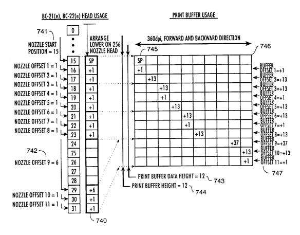
[BC-21(e) OR BC-22(e) 24 NOZZLE OF COLOR, 720dpi, FORWARD AND BACKWARD] (LOWER 3 BYTE IS USED FOR BLACK) PRINT BUFFER USAGE
