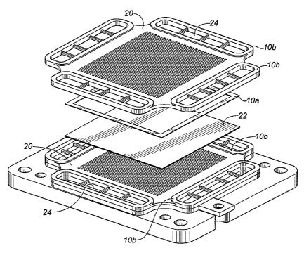
(57) Abstract: A flexible seal for use in a solid state oxide fuel cell stack is formed from a fibre matrix impregnated with a plurality of solid particles. The fibres and particles are preferably ceramic and may be formed from alumina or zirconia. The seal may be formed by dipping the fibre matrix into a slurry of the particles in an alcohol, drying the seal and precompressing prior to installation in the fuel cell stack.
