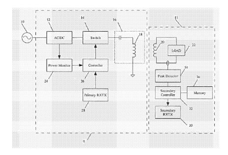
(57) Abstract: An inductive power supply includes a transceiver for sending information between the remote device and the inductive power supply. The remote device determines the actual voltage and then sends a command to the inductive power supply to change the operating frequency if the actual voltage is different from the desired voltage. In order to determine the actual voltage, the remote device determines a peak voltage and then applies a correction factor.
