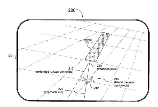
(57) Abstract: Systems and methods to accurately display lateral deviation symbology in offset approaches to runways is provided. A system for on-aircraft display of lateral deviation symbology for use in offset approaches comprises means for generating a conformal video display representation of an aircraft's current position, means for notifying a flight crew of the existence of an offset approach, means for displaying an extended runway center line, and means for displaying an approach line.
