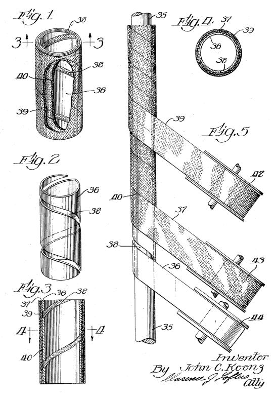
HEAT DISSIPATOR FOR ELECTRICAL DEVICES AND EQUIPMENT
