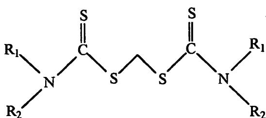
where R<sub>1</sub> and R<sub>2</sub> may be the same or different alkyl groups of from 1 to 12 carbon atoms and preferably R<sub>1</sub> and R<sub>2</sub> are the same and have four carbon atoms.
