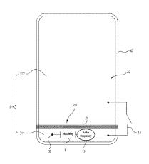
achieved by the metal rear cover, when the conducting switch disconnects or connects the first radiation part with the second radiation part.
