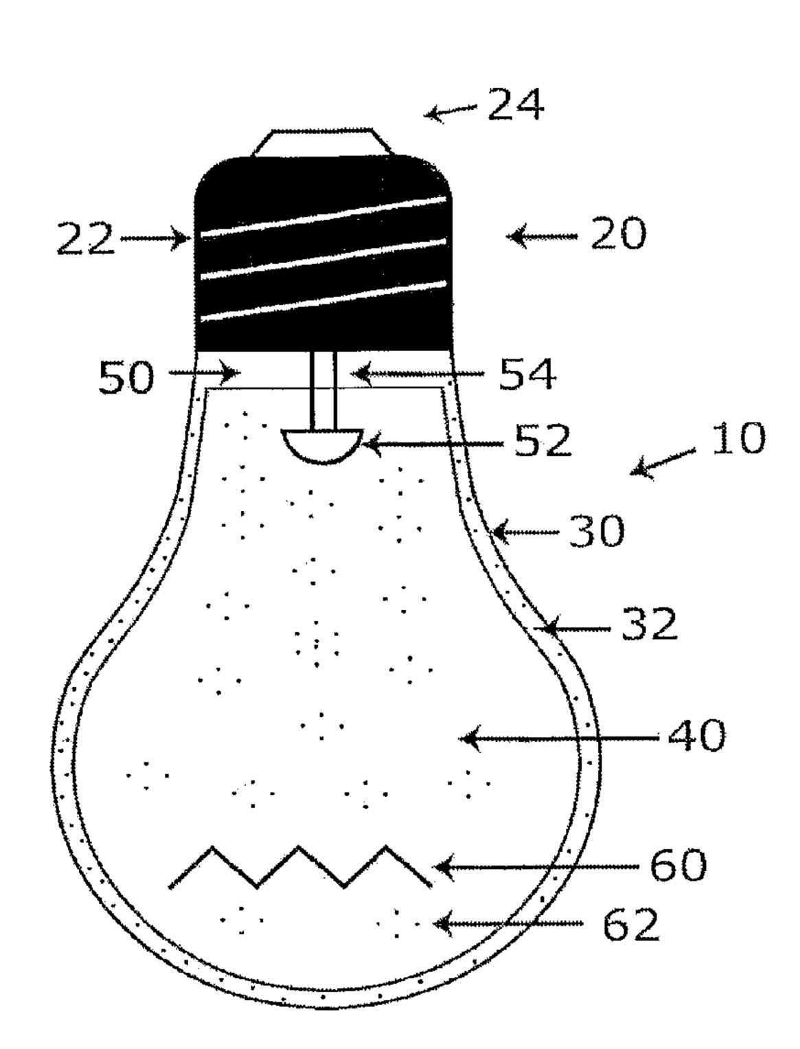
(57) Abstract: An LED bulb having a bulb-shaped shell, a thermally conductive plastic material within the bulb-shaped shell, and at least one LED within the bulb-shaped shell. The bulb also includes a base, wherein the base is dimensioned to be received within a standard electrical socket.
