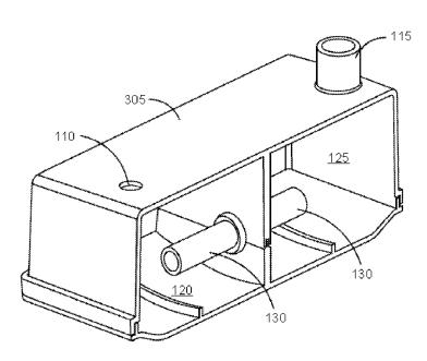
(57) Abstract: A device combines a muffler and a filter such as for use with an air compressor. The device utilizes dual expansion chambers with an internal connecting tube to filter the air entering an air intake port of an air compressor or oxygen concentrator. The device attenuates sound that emanates from airflow through the chambers
