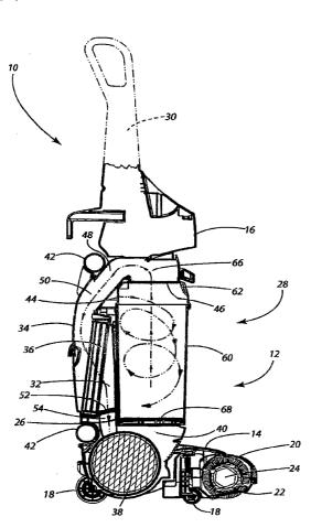
(57) Abstract: A vacuum cleaner includes a housing as well as a suction generator and bagless dirt system carried on the housing. The bagless dirt system includes a dirt cup, a prefilter, a filter chamber remote from the dirt cup, a filter in the filter chamber and a first conduit providing fluid communication between the dirt cup and the filter chamber. A second conduit provides fluid communication between the filter chamber and the suction generator.
