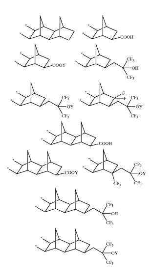
**[0027]** Preference is given to using resists with polymers where the polymer contains repeating units which contain carboxylic anhydride groups or bicyclic or polycyclic aliphatic groups. Particular preference is given to copolymers of cycloolefins and maleic anhydride, which are present as the polymer in what are known as COMA resists.
