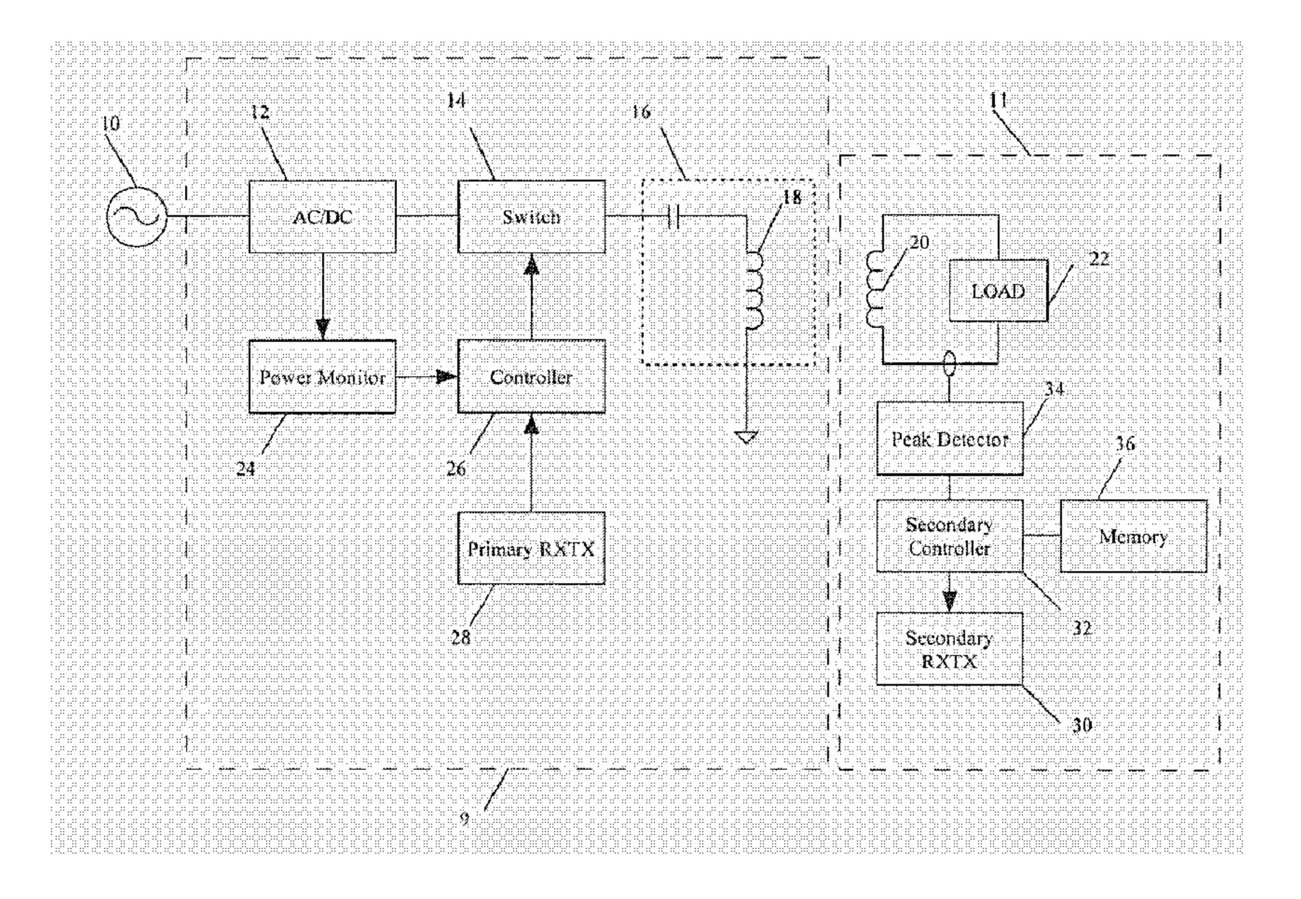
(57) Abstract: An inductive power supply (9) includes a transceiver (28) for sending information between the remote device (11) and the inductive power supply. The remote device determines the actual voltage and then sends a command to the inductive power supply to change the operating frequency if the actual voltage is different from the desired voltage. In order to determine the actual voltage, the remote device determines a peak voltage (34) and then applies a correction factor.
