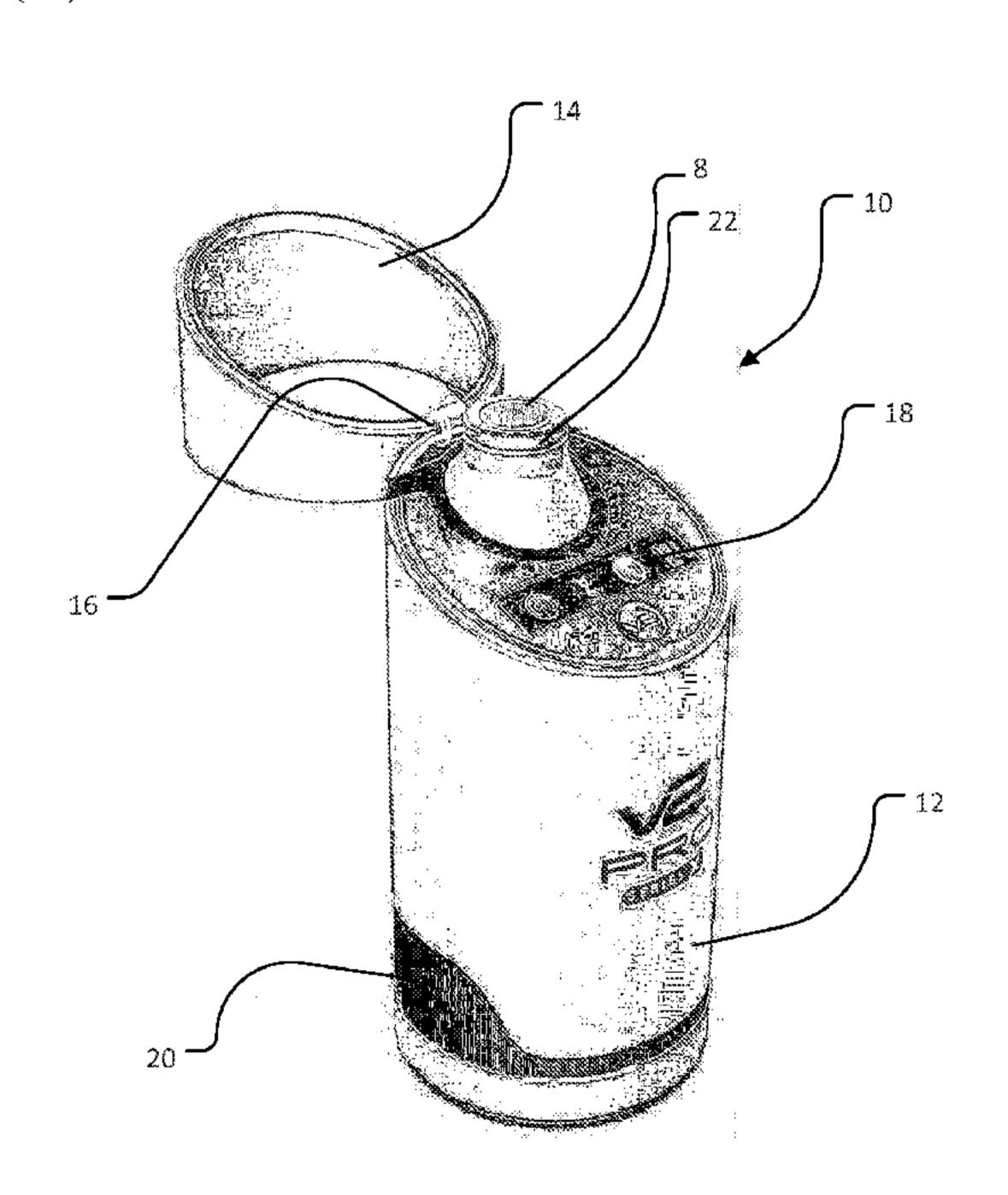
ber (38), an air channel (34), and a control panel (18). The control panel is in electrical communication with a battery (24), the air pump, and the heating block and is configured to control a speed of the air pump and a temperature of the heating block.
