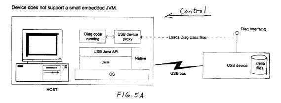
NOTE: Once the device enumerates it exposes an interface which allows the host to load the Java class files (executable Java byte code). The host then sets up a device proxy which it uses to perform the functions described above, including diagnosing the USB device.
