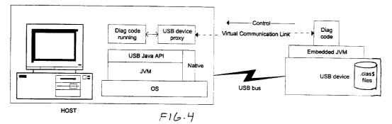
NOTE: Once the USB API is ported over the different Java supported platforms, then this scheme works independently of the underlying OS. The USB API can be considered as a standard extension to the Java API.
