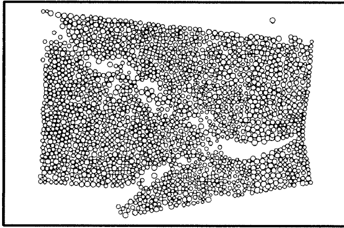
Cylinder that Experienced a Brittle Failure
