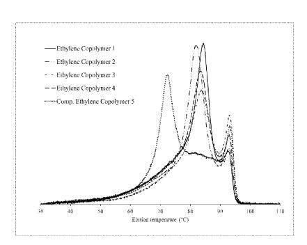
(57) Abstract: Ethylene copolymers made in the gas phase using a phosphinimine based single site catalyst supported on a passivated inorganic oxide support. The ethylene copolymers have a relatively narrow molecular weight distribution and good rheological parameters.
