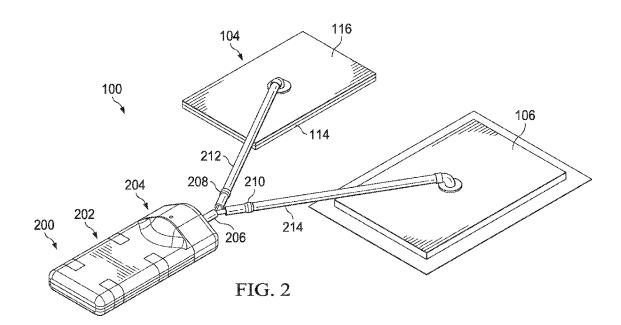
(57) **Abstract:** An apparatus for negative-pressure treatment may include an enclosure having a variable volume, a port and an actuation surface, a first one-way valve configured to allow fluid ingress to the enclosure, a second one-way valve configured to allow fluid egress from the enclosure, and an actuator configured to apply a linear force to the actuation surface.
