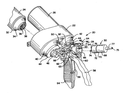
(57) Abstract: A chemical product dispenser (20) and a manifold (50) attached thereto. The manifold (50) includes two separate passages (110), (118) for directing the contents from two pressurized valved containers (24), (26). The manifold (50) includes two adapters (46), (48), each having a different structural configuration that can only be secured to a correspondingly matched containers intended to be attached thereto.
