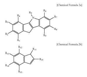
[0035] in Chemical Formula 2a,  $R_1$  to  $R_9$  are the same as or different from each other, and each independently hydrogen, a C1 to C20 alkyl group, a C2 to C20 alkenyl group, a C1 to C20 alkoxy group, a C1 to C20 alkylsilyl group, a C1 to C20 alkylsilyl group, a C1 to C20 alkylagroup, a C7 to C20 aryl group, a C7 to C20 alkylaryl group, or a C7 to C20 arylalkyl group;
