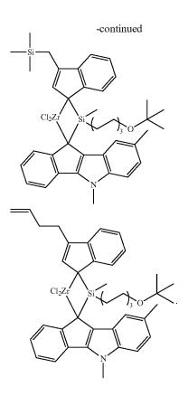
**[0055]** The metallocene compound may have an excellent activity and may polymerize an olefinic polymer having a middle molecular weight to a high molecular weight.
