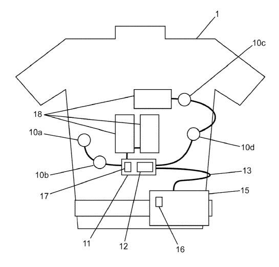
Figure 2: System diagram with accelerometers
