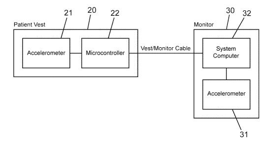
**Figure 3: Monitor Accelerometer**
