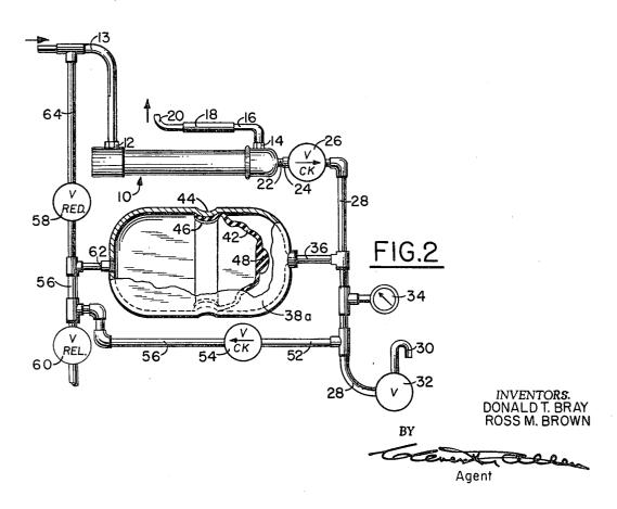
PURIFIED WATER SUPPLY APPARATUS AND METHOD
