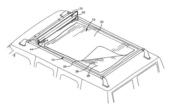
(57) Abstract: A retractable carrier system (10) is provided for carrying luggage and other objects on the roof of a vehicle. The carrier system (10), which may be original equipment on the vehicle or an after market addition, includes a collapsible container (20), a reel (50) onto which the collapsible container (20) may be rolled and a storage compartment (70).
