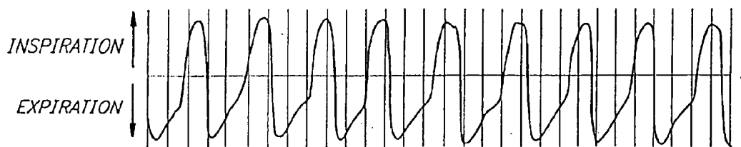
FIG. 1 AIRFLOW TO AND FROM CPAP GENERATOR
