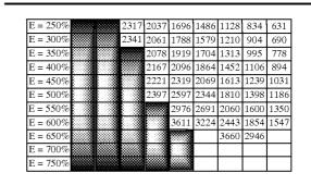
Table 5: Stress versus extension (E) data for blends of first polymer component and second polymer component where the second polymer component is component SPC-2 in the tables above. Shaded areas with no data represent broken samples. Clear areas represent lack of data due to extension beyond machine limits.
