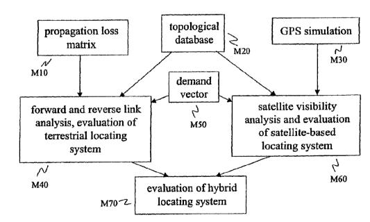
(57) Abstract: Several different approaches may be taken to adding mobile unit position location capability to a system for wireless communications. These approaches may include terrestrial techniques as well as satellite-based techniques. An apparatus is disclosed whereby different such approaches may be evaluated and compared in the context of a particular existing or proposed system for wireless communications.
