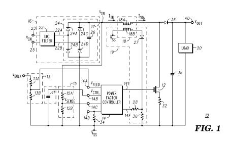
(57) Abstract: In accordance with an embodiment, a converter includes a power factor controller that varies the switching frequency of a switching transistor in accordance with a signal representative of power at the input of the converter.
