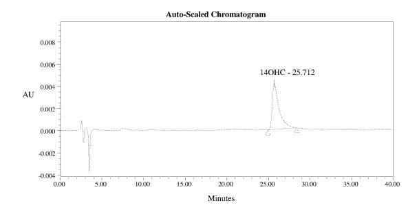
Typical HPLC Chromatogram of the Sample Solution containing Oxycodone API
