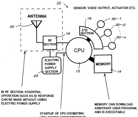
STARTUP OF CPU EXHIBITING HIGH POWER CONSUMPTION IS CONTROLLED BY RF SECTION
