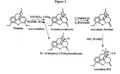
Reaction scheme of the process used to produce oxycodone HCl from thebaine.
