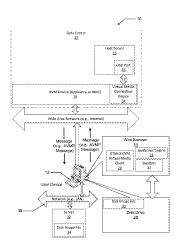
virtual media client exposes the disk image file for use to the remote device, which sends a message to the HTML5 KVM virtual media client requesting a specific portion of the disk image file. The HTML5 KVM virtual media client receives the message and a script engine running in the Web browser creates a new file available to the Web browser of just the portion requested by the remote device, which is then transmitted to the remote device.
